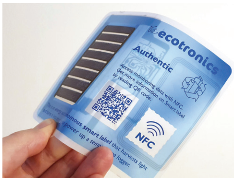
VTT and university partners have integrated a thin and flexible electronic label for condition monitoring based on bio-based and environmentally friendly materials.
